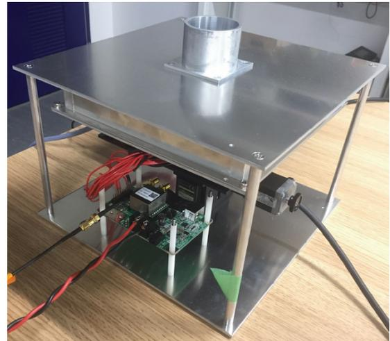
Figure 3. A photo of the developed camera system with the FPGA evaluation board.
